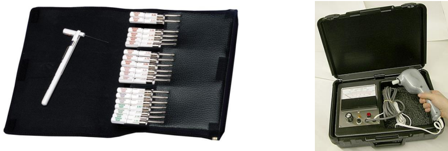
Figure 8. The Touch Test™ Sensory Evaluators, Semmes-Weinstein Von Frey Aesthesiometers (right) and Bio-Thesiometer (left).
