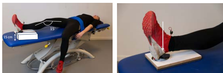
Figure 16: Isometric strength tested with a handheld dynamometer (microFET 2; Hoggan Health Industries). Handheld dynamometers can be used in many different settings. In Studies 2 and 4, the patient was placed in the supine position with the heel on a 15 cm box and the knee in 15 degrees of flexion. The patient was instructed to apply a maximum contracting force at the dynamometer for 1-3 seconds. The maximum force in N was recorded.
