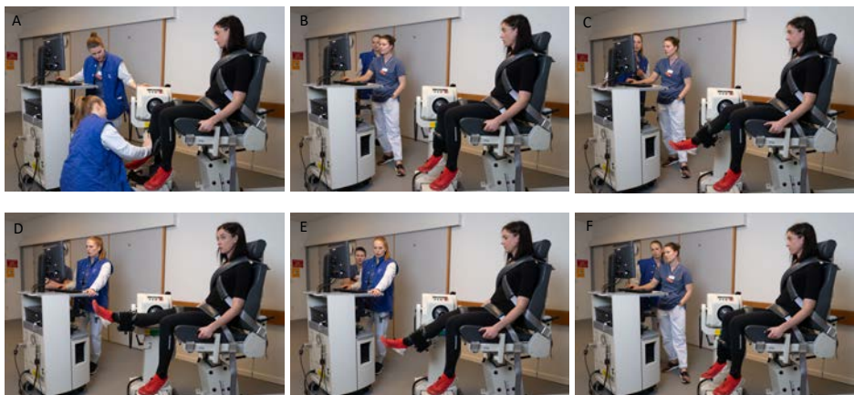
Figure 15: Isokinetic strength test measured with a Biodex Pro System 4 dynamometer (Biodex Medical Systems, Inc.). Patients can be positioned following a predetermined protocol (A), allowing for individual adjustment of, e.g., range of motion. When the dynamometer extends the leg, the patient should try to resist this force (C), and when the dynamometer allows flexion, the patient should try to contract against the by the dynamometer applied resistance (E). Different speeds of the dynamometer can be applied, and the peak torque (N) or total workload joule (J) can be recorded. The isokinetic strength test was used in Studies 2 and 3.
