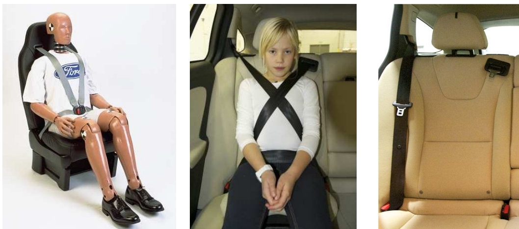
Figure 8 a) A four-point belt system presented by Ford (Courtesy of Ford). b) Shows a prototype of a five-point belt system (criss-cross pattern) with a child occupant in the rear seat of a mid-sized vehicle (Autoliv 2013). c) Shows a prototype of a five-point belt system in the rear seat of a mid-sized vehicle (Autoliv 2013).
