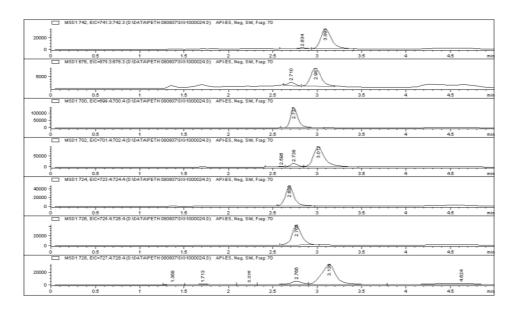
Fig. 4. An LC-MS chromatogram of an extracted PEth positive whole blood sample. In SIM, PEth molecules with identical masses are not separated but measured as a single peak. For example, PEth-16:0/20:3 and PEth-18:1/18:2 share a common molecular mass of m/z 725.6.
