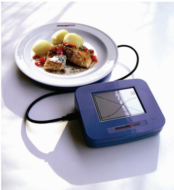
**Figure 2.** Mandometer<sup>®</sup>, a personal computer connected to a scale recording the weight loss of a plate during the meal. Feedback on how to eat can be provided on the touch screen.
