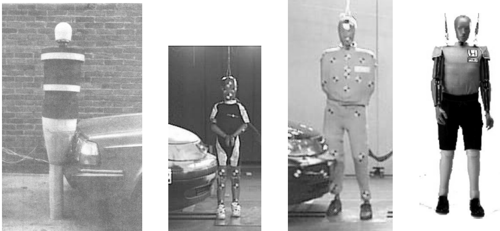
Figure 5. Pedestrian dummies (from left): Aldman et al. rotationally symmetric, Autoliv/Chalmers child and adult dummies, Polar II
