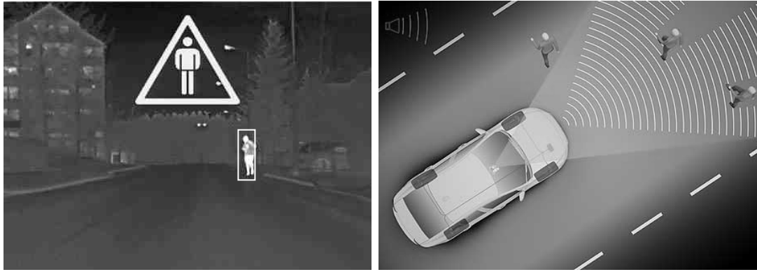
Figure 8. Primary pedestrian safety systems; (driver display of) pedestrian warning system (left), auto-brake system detecting pedestrians at danger (right)
