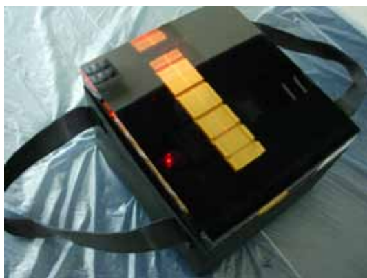
FIGURE 48. Aluminum phantom used for weekly accuracy calibration. Photo by Hans-Jerker Lundberg
