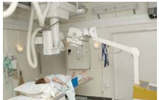
FIGURE 44. RSA setting in Study IV showing the fixed and the mobile x-ray tubes.
