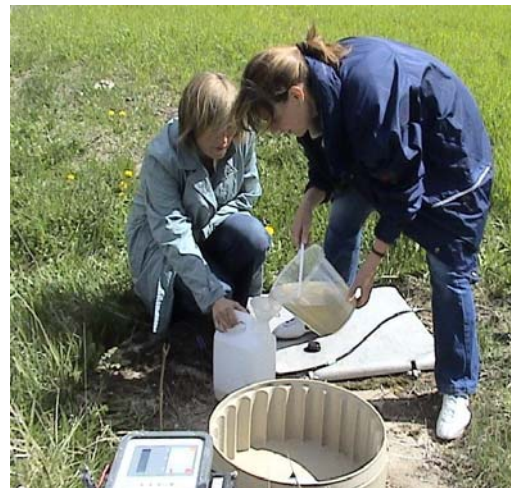
Figure 4. Time proportional collection of sewage, from the anthroposophic village Järna, using a sampler
