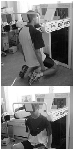
Figure 8. Test position for measuring isometric neck maximal voluntary contraction (MVC) in extension (upper picture) and flexion.
