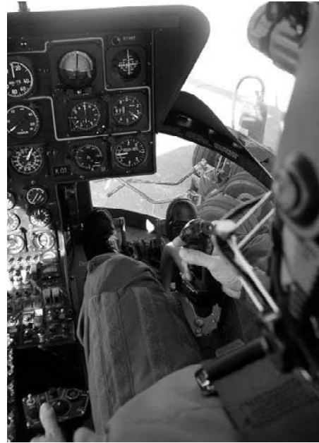
Figure 2. Helicopter pilot seated in the cabin with right hand on cyclic flight stick and left hand on collective stick. Feet continuously control the rudder pedals, thus no fixed support under the feet, i.e. sitting in an open-chain situation.
