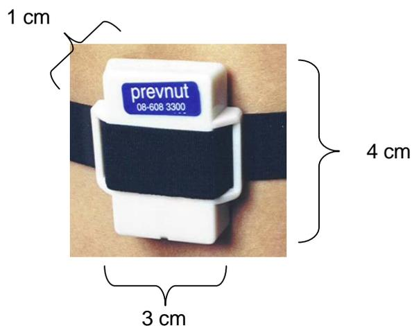
**Figure 5.** An example of an accelerometer, worn at the lower back.
