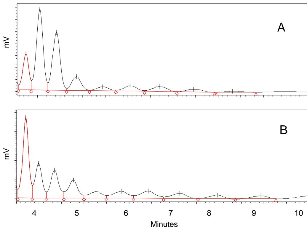
**Figure 3.** Chromatograms of a plasma sample (A) from a patient using icodextrin solution and a dialysate effluent sample (B). The first peak to the left correspond to glucose, followed by maltose (G2), G3, etc.
