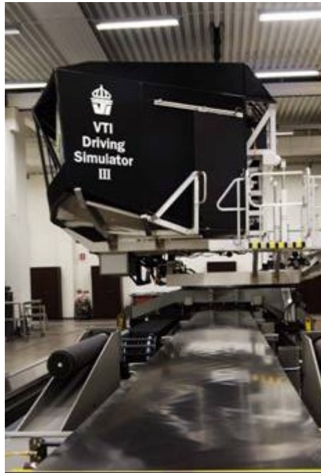
Figure 4 Moving base driving simulator (version III) at VTI, Sweden.
