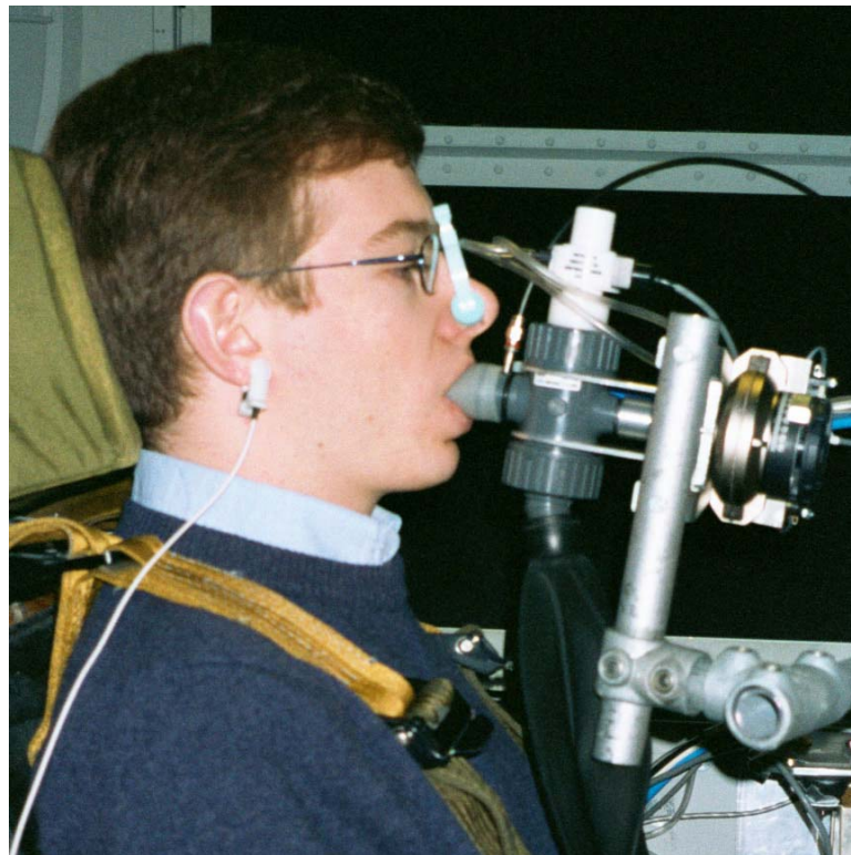
Fig. 3. A seated subject and parts of the experimental setup (Papers II and III). Note that the flow meter is placed in a different position from that in the experiments and in Fig. 4.
