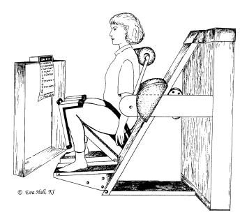
**Figure 3.** Subject in position for isometric trunk extension. A display unit in front of the subject continuously showed the applied torque.
