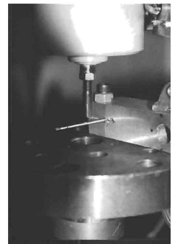
Figure 6: Bone pin undergoing mechanical testing (study IV).
