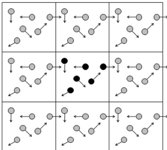
**Figure 13. Periodic boundary conditions in two dimensions. The real system is in the center with black circles.**
