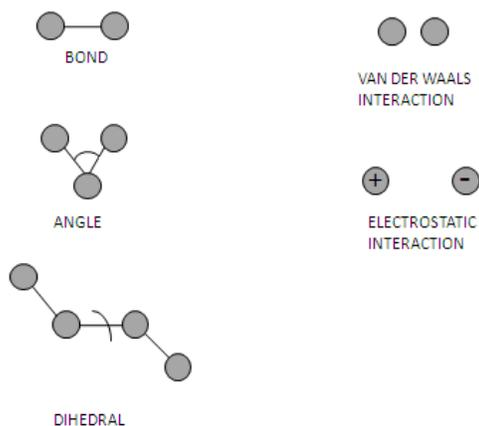
Figure 12. Interactions in the potential energy function in MD simulations.
