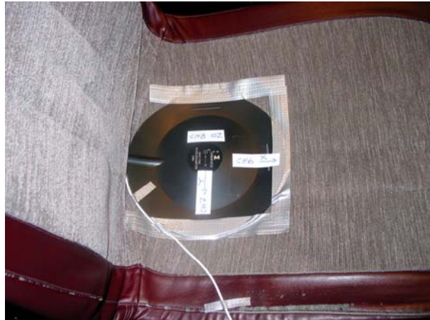
Figure 6. Tri-axial seat accelerometer positioned in helicopter seat.
