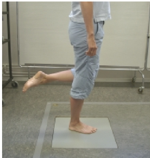
Fig 6. Measurements of postural control on an AMTI ® force platform (model LG6-4-2000, Advanced Mechanical Technology, Inc., Watertown, MA, USA)
