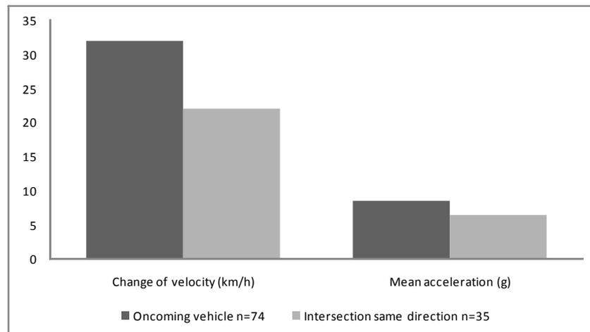
**Figure 13.** Measured change of velocity and mean acceleration in frontal crashes for the two most severe crash types.
