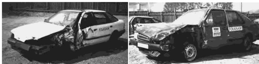
**Figure 24.** Left vehicle with interior intrusion – right vehicle no intrusion. (Kullgren et al., 1998)
