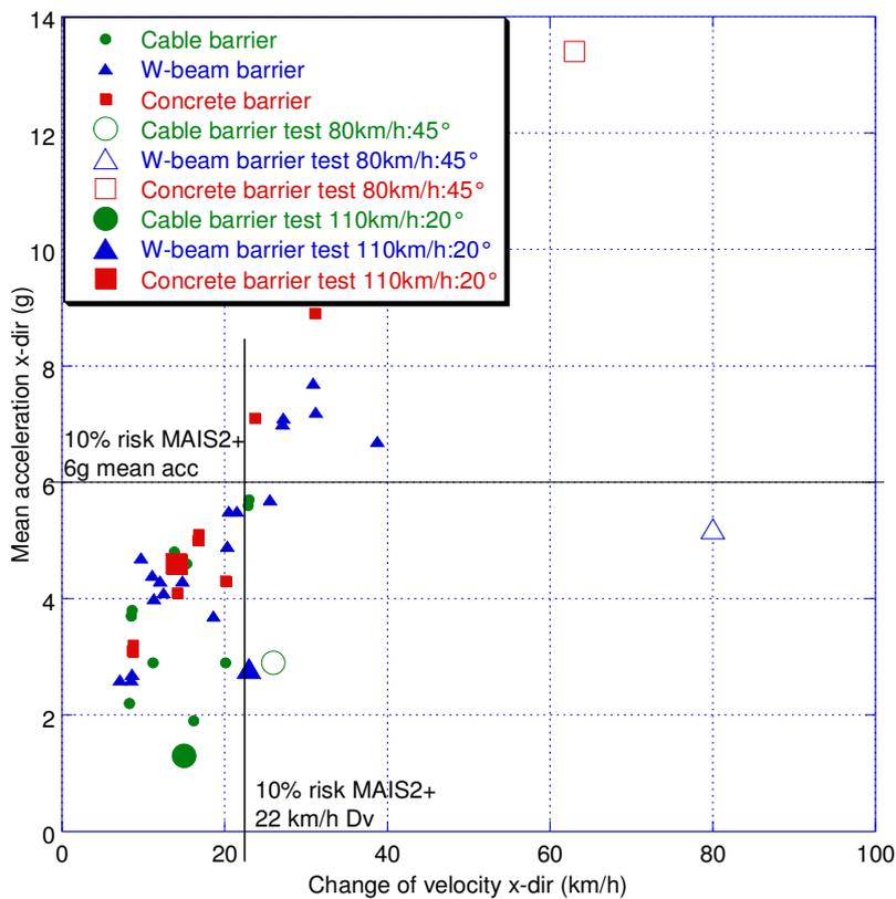
**Figure 26.** Real-world guardrail crash impacts (n = 37) and guardrail tests (n = 6) from Study IV.
