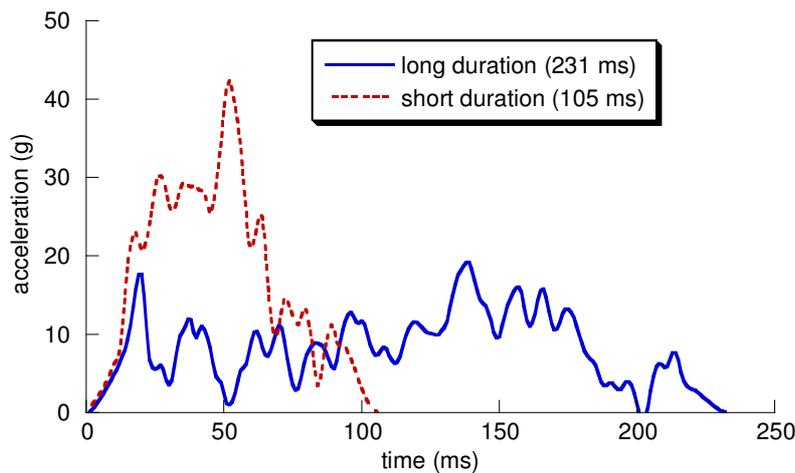
**Figure 22.** Two crash pulses with same change of velocity and different pulse duration. Source: Study III
