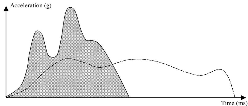
**Figure 25.** Crash pulse with similar change of velocity and different duration.
