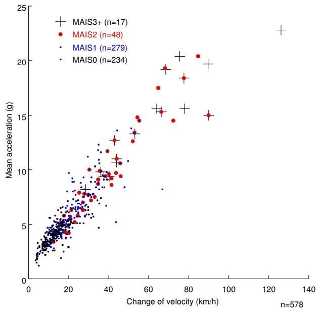
**Figure 20.** Correlation between change of velocity and mean acceleration
