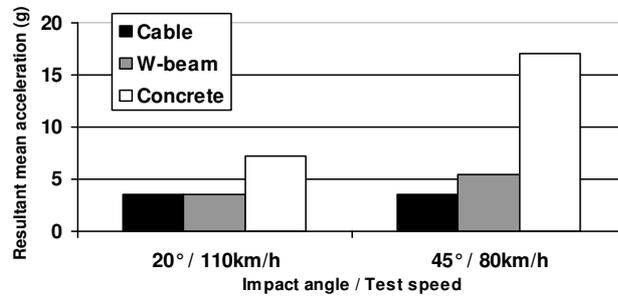
**Figure 21.** Resultant mean acceleration measured in guardrail crash test.
