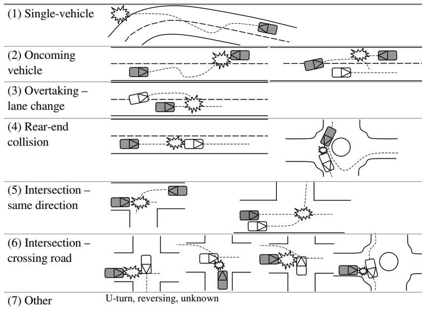
**Figure 12.** Crash types divided according to SIKI. Dark vehicle with measured crash severity.
