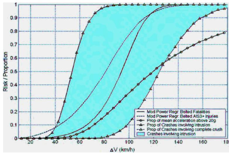
**Figure 11.** Distributions of onset of intrusion, complete car crush and mean acceleration above  $20\times g$  compared to real world belted driver AIS3+ and fatality risk functions. Wood et al. (2007).
