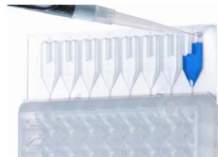
**Figure 4.** Loading of TLDA card [1].
