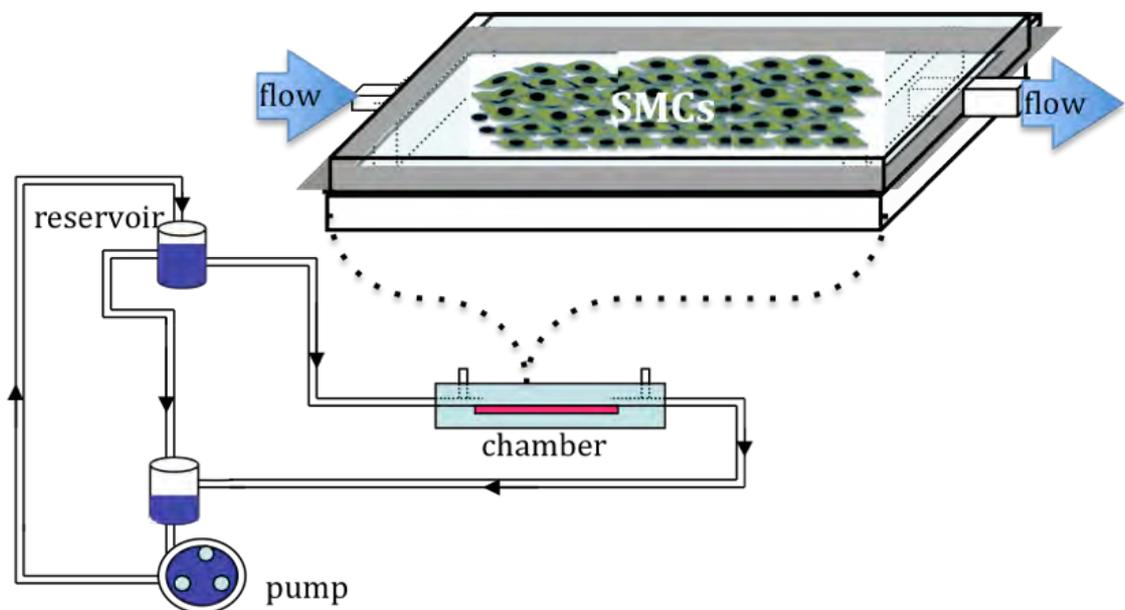
**Figure 7.** Model of the parallel plate flow chamber.
