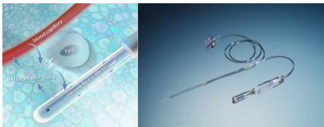
Figure 10A-B. The principles of the microdialysis (A) and the CMA 71 microdialysis catheter (B), published with courtesy by MDialysis AB.
