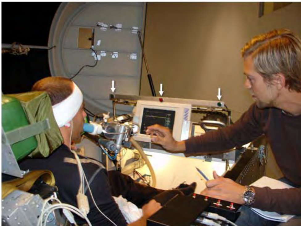
Figure 13. Seated subject in the gondola of the human centrifuge during a 1 G control test. Arrows show lamps for monitoring of peripheral vision.
