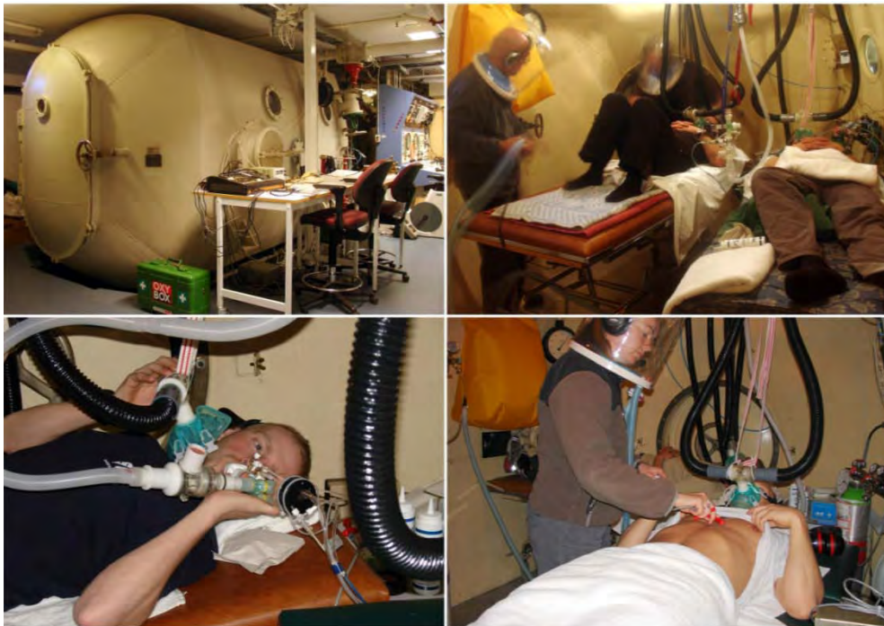
Figure 9. Upper left panel: hypobaric pressure chamber at Karolinska Institutet. Upper right panel: inside view of the hypobaric pressure chamber with two subjects and two attendants. Lower left panel: subject exhaling into equipment to determine exhaled nitric oxide. Lower right panel: Doppler ultrasound monitoring of venous gas emboli passing the subjects heart.
