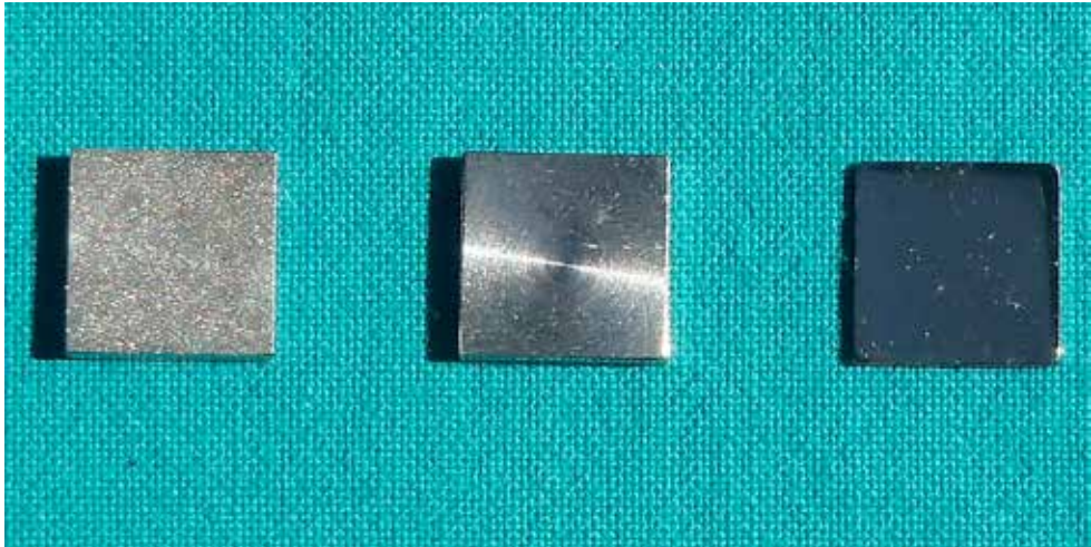
Figure 17: Three degrees of roughness from left to right; sandblasted, original, mirror glossy.
