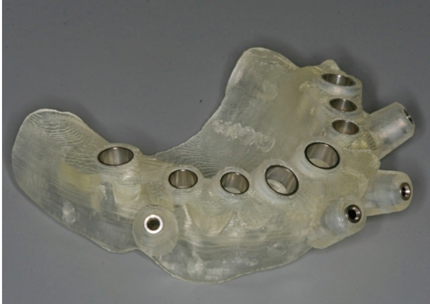
Fig. 12. NobelGuide, CAM produced surgical template.
