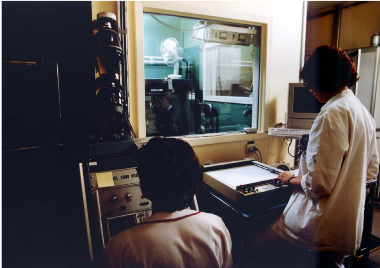
Figure 3. NO 2 exposure chamber.
